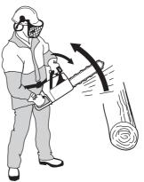
If the kickback is less violent or the kickback zone of the bar is closer to you the chain brake is designed to be activated manually by the movement of your left hand.
